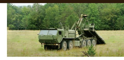
Cab Seating: 2 person Axle Configuration: 10×10 Curb Weight: 53,700 lbs. (24358 kg) Gross Vehicle Weight Rating (GVWR): 106,000 lbs. (48081 kg) Length: 431 in. (10947 mm) Width: 98 in. (2489 mm) Height: 139 in. (3531 mm) Reducible Height: 102 in. (2591 mm) Track: 81 in. (2057 mm) Wheelbase: 223 in. (5664 mm) Maximum Speed: 65 mph (105 km/h) Tires: 16.00 R20 XZL Michelin tubeless Number of Tires: 10
